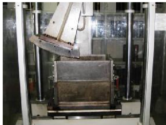
Fig. 25: Laboratory Roller Compactor according to DIN EN 12697-35
