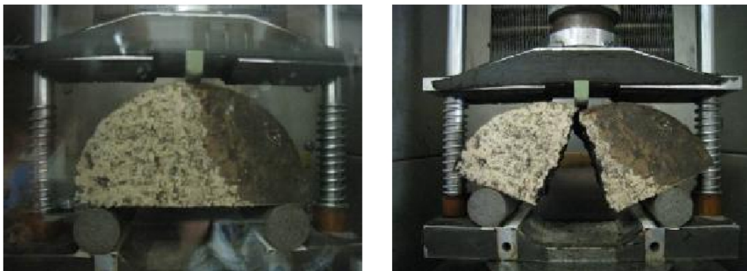
Fig. 1: EN 12697-30 Marshall-Test Stability, Flow and Marshall Quotient Value
