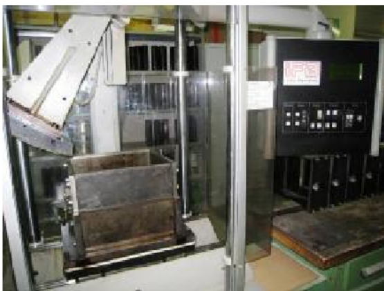
Fig. 25: Laboratory Roller Compactor according to DIN EN 12697-35
